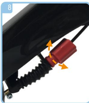
To adjust the braking strength, adjust the brake by pressing the screw housing downwards and then turn left or right (picture 8).
