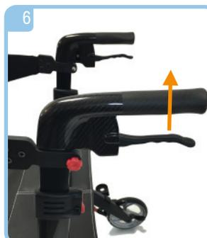
Pull both brake levers upwards to apply the brakes whilst the rollator is moving (see picture 6). Always brake slowly and steady.
